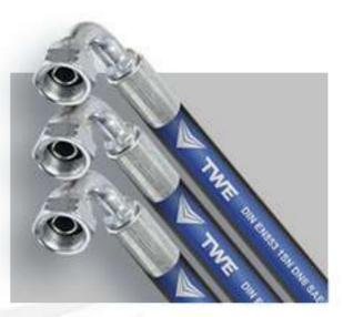
When this braid is high tenacity brass-plated steel wire, this hose can be used for medium and high pressure. This type of reinforcement can have from one to three layers, and always separated by a layer of adhesive rubber to avoid friction between the layers.
